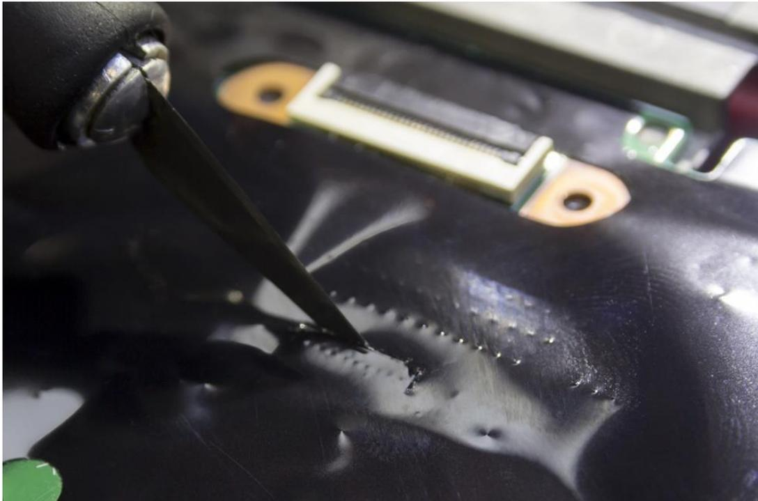
Figure 3. Removing the protective film (cutting edge points up)
