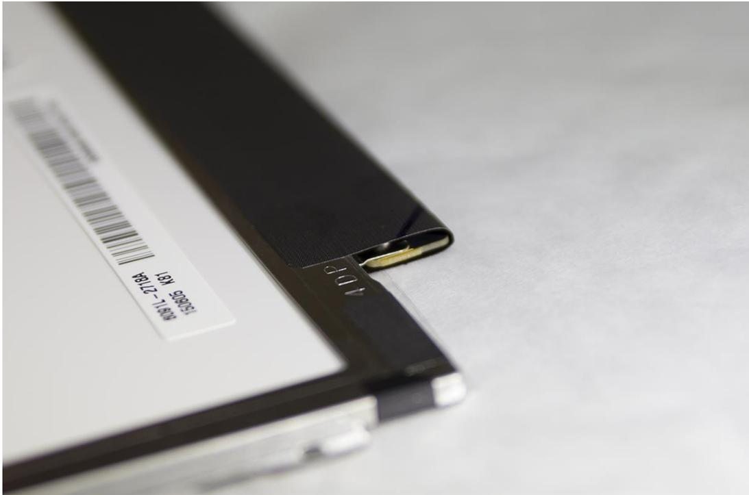
Figure 22. The logic board (dark line on the protective cover shows the required corner shape)
